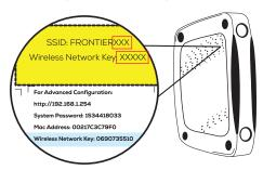
Connect wirelessly with a wireless-enabled notebook or a computer with an 802.11b/g/n/ac wireless network adapter installed.
